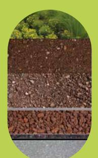
Procedure according to FLL Intensive multi-layer greening
