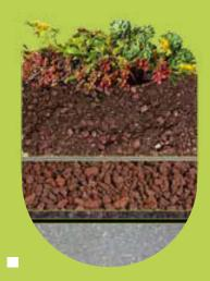
Procedure according to FLL Extensive multi-layer greening
