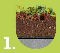
Procedure according to FLL Extensive mono-layer greening
